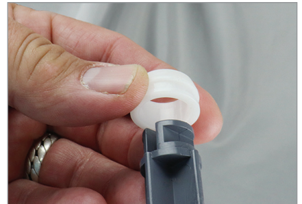
3. Place retainer ring on adjustment tool.
