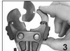
3. With the side release spring pressed upward, slide new jaw into place and release the spring.
