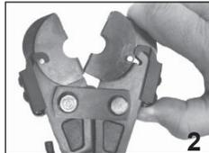
2. Slide jaw out of position and remove.
