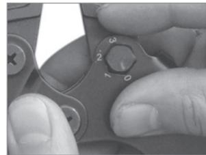
3. Push the screw back into place and tighten the nut.
