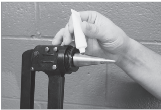
1. Lightly grease the cone of the expansion tool.
