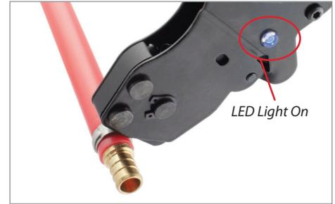
3. Place pinch clamp nub between tool jaws and ratchet the clamp (approximately seven times) until the LEDlight comes on. This will assure that the pinch clamp is fully engaged.
