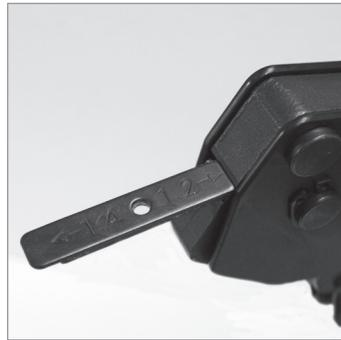
2. Use the Calibration Tool to gauge the jaw gap. The jaw gap should be between 1.2 mm and 1.4 mm.
