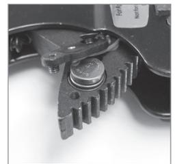
5. Place the new batteries with the positive side facing up. Replace the cover and tighten the screws.
